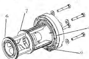
3 - No Hard Water Bypass Valve Cartridge
