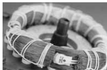
Fig. 47 Thermal switch incorporated in windings
