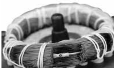
Fig. 45 PTC sensor incorporated in windings
