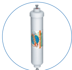
2" x 10" in-line cartridge with NSF approved coconut shell granulated activated carbon (GAC) - 1/4" QC. activated carbon (GAC) and bacteriostatic polypropylene fiber - 1/4" NPT.
